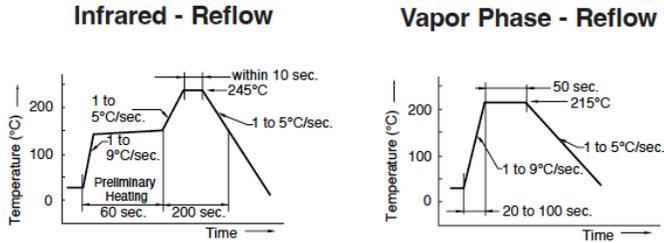
Figure E) Time Temperature Profiles
